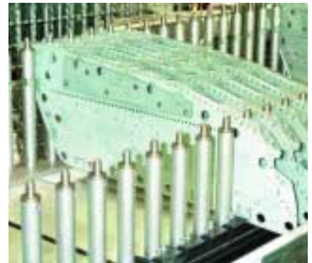
Pallet-conveyor with steel inserts, positioned
