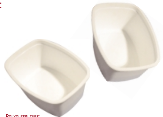
POLYOLEFIN TUBS: • THIN-WALL APPLICATION OF 40 MFI POLYOLEFIN MATERIAL • WALL THICKNESS - 0.5 MM (0.020") • ELIMINATION OF HOLD AND COOLING TIME • FLOW RATIO = 280:1 • 10% MATERIAL REDUCTION
